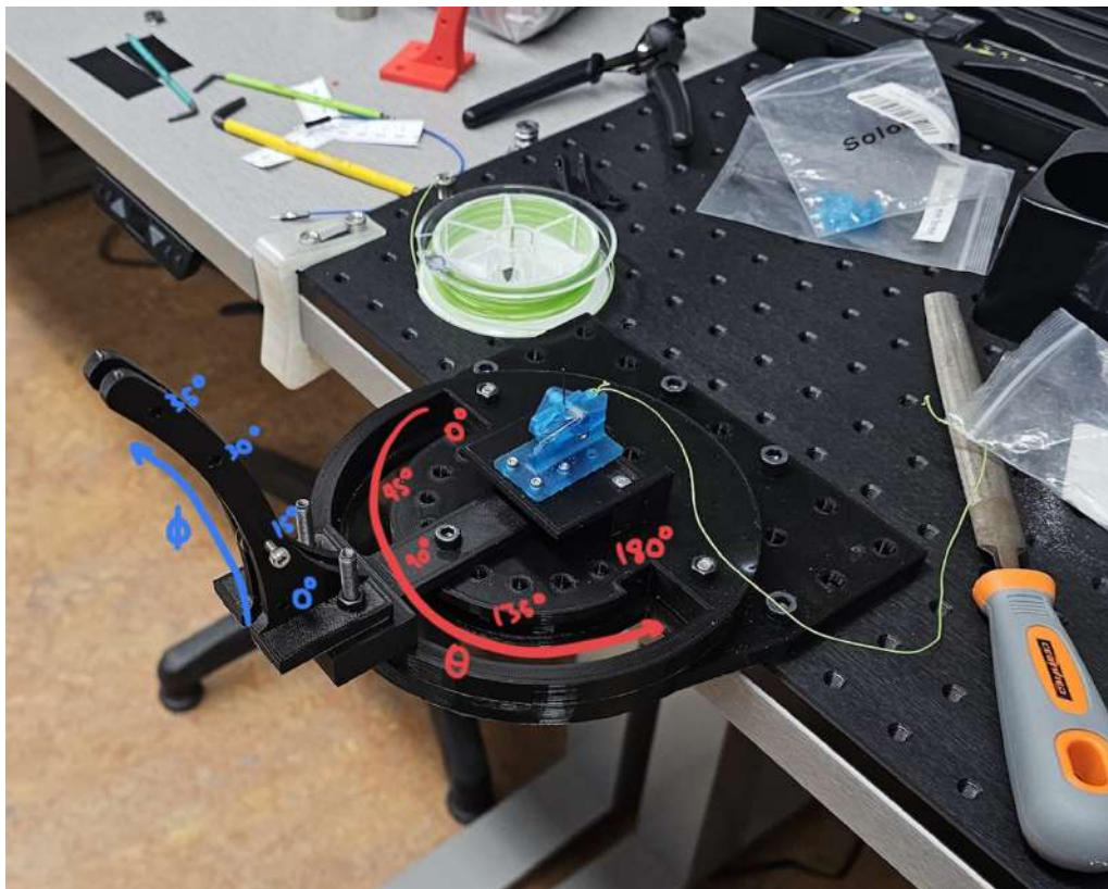
Figure 32: Labelled image of the 2 DOF testing mechanism.
