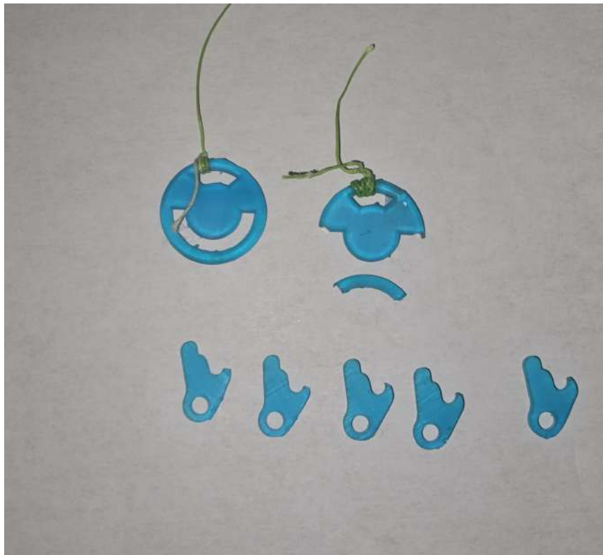
Figure 44: Samples of failed latches and failed disks.
